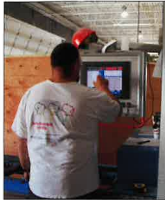
Alpine Linear Saws are among the manufacturing equipment in the CCC plant that are computer-controlled and driven by VIEW design software.
