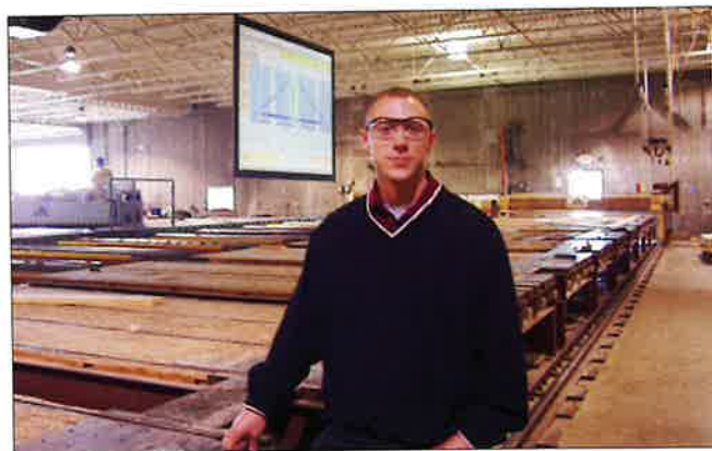
The 8 x 12-foot image projected on the screen behind Plant Manager Eric Goratowski is an integral feature of the eShop system. It provides an easy reference for the table crew. Eric says CCC plans to replace the projector with large flat-panel monitors located above each assembly table station.
